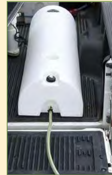
IBC totes (above) carry 110 to 275 gallons of water while a laydown tank (right) holds about 48 gallons. Both can be carried in the bed of a pickup truck.
